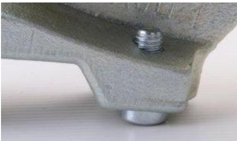
Picture 2 Screws must be at the same level
